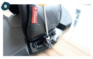
The Geek Pads are fully adjustable to fit a variety of foot sizes, shapes, and comfort levels, thanks to it multiple velcros. Make sure you experiment with the settings and find what works best for your foot size and riding style.
