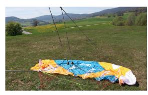
Ensure that your flying lines are correctly connected and that you are clear of any potential risks. Make sure there are no damages or knots.
