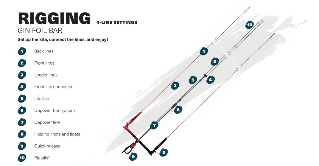
For the Marabou 2, the Gin Bar and the Gin Foil Bar are recommended. The 52cm size is for 4 to 8m² kites, and the 60cm is more suitable from 10 to 12m². In terms of line length, we recommended using 17m from 4 to 8m² and 19m from 10 to 12m².
