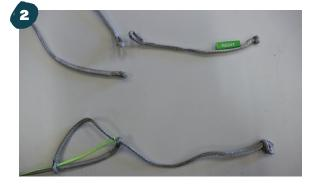
Disconnect the rest of the speed system and identify the parts to be changed. Replace worn parts.
