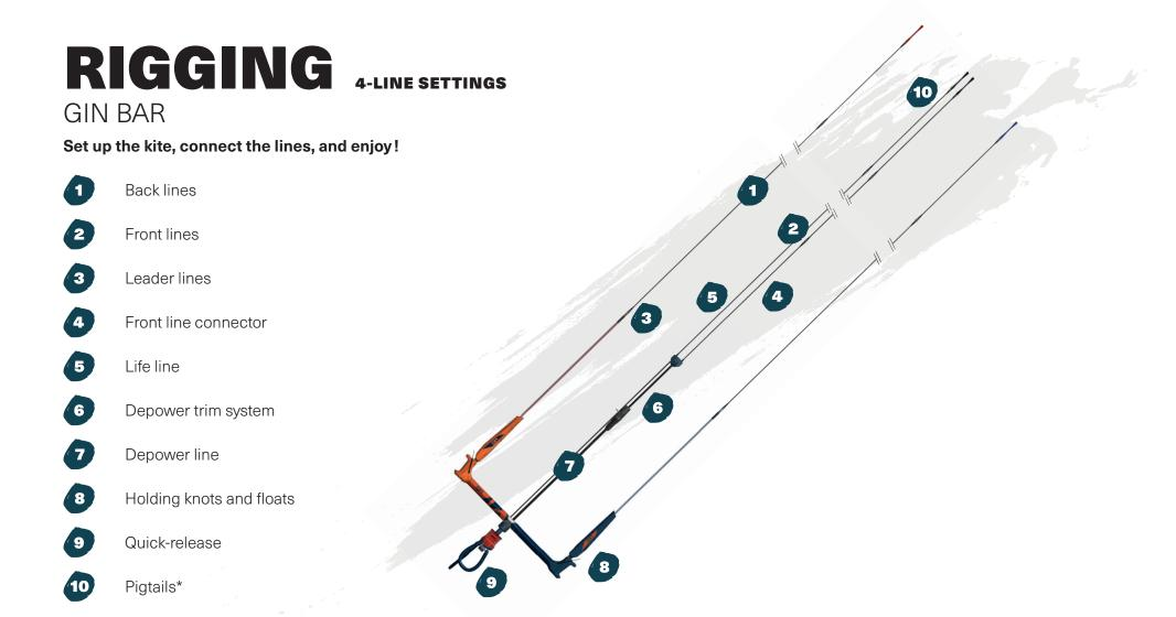
For the Marabou 2, the Gin Bar and the Gin Foil Bar are recommended. The 44cm size is for 4 to 8m² kites, and the 52cm one is more suitable from 10 to 12m². In terms of line length, we recommended using 19m.
